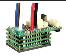
The **FXM060-25-EM** is an Extended Environment single-axis servo drive and integration board assembly for a FXE060-25-EM FlexPro<sup>TM</sup> series servo drive with IMPACT<sup>TM</sup> architecture. Connections to the controller, motor, power, and feedback are simplified through the standard connectors featured on the board.
